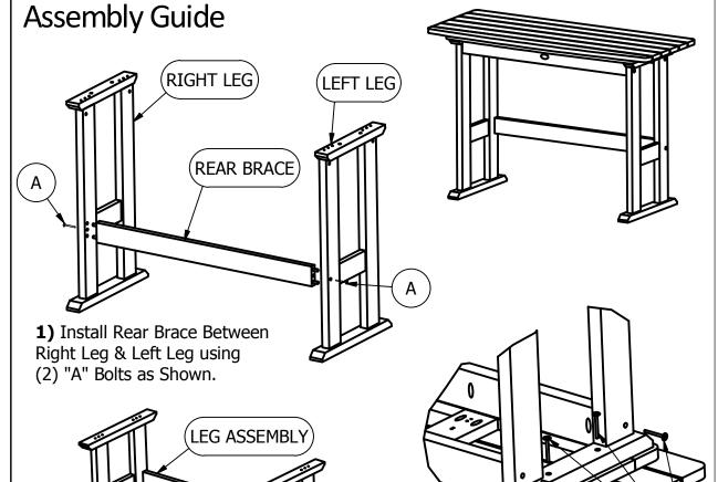
**2)** Turn Leg Assembly Over and Set on Table Top as Shown. Attach Leg Assembly to One Side of Table Top Using (4) "A" Bolts. Repeat on Other Side.
